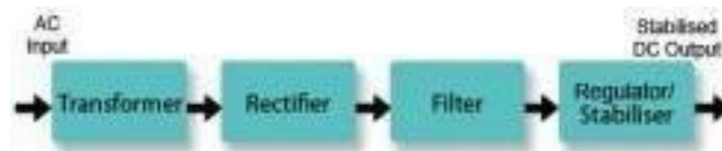
Figure 7: Block diagram of a fixed regulated power supply
